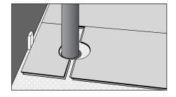
For a double pipe, drill a hole equivalent to the diameter of the pipe plus 1/2 inch (13 mm) at each of the marked points. If located on the long side of the plank, make a 45° cut from each hole to the edge of the plank. Apply Sealer along the cut edges of the piece you cut out, seal the piece in place. Be sure no sealer comes between the cut-out piece and the subfloor.
